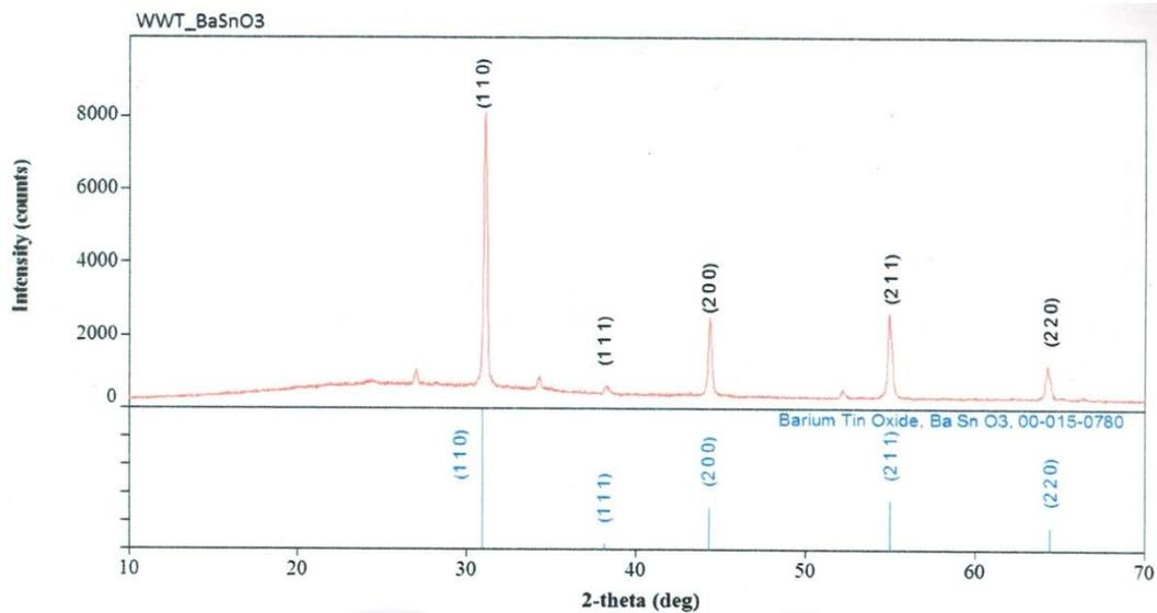
**Figure 3** XRD pattern of BaSnO<sub>3</sub> film sample
