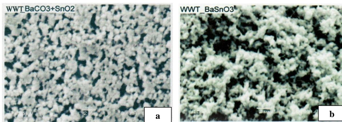
**Figure 4** SEM micrograph of (a) BaSnO<sub>3</sub> powder sample (b) BaSnO<sub>3</sub> film sample
