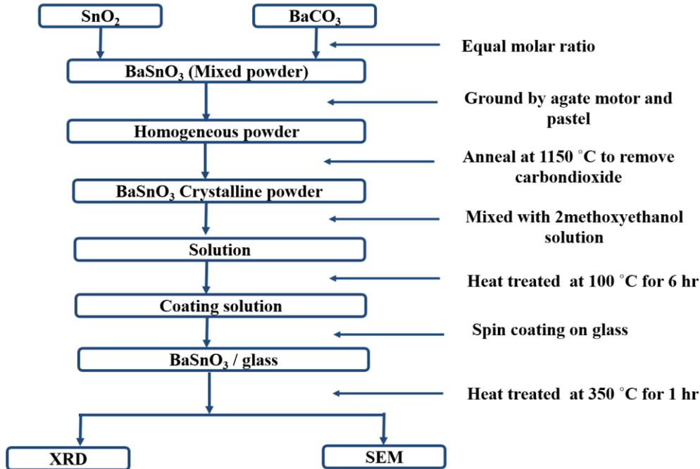
**Figure 1** Flow chart of the preparation of BaSnO<sub>3</sub> sample
